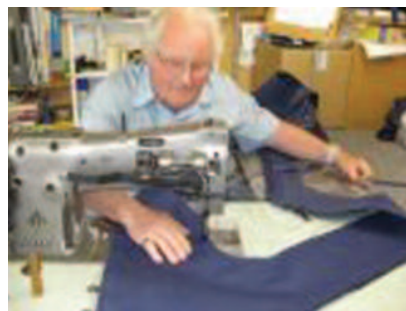
Above: Mike working on a yacht's sprayhood to protect the crew in the boat's cockpit. Right: his distinctive 'label' and, below: a spray-hood and sail cover on a boat at Levington.
